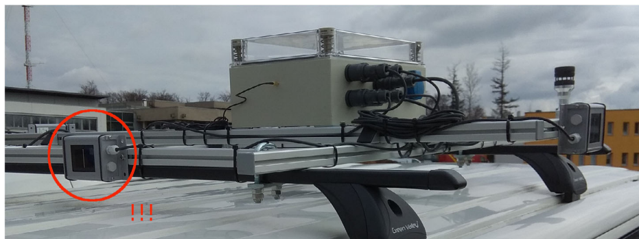
Figure 1. View on the sensor box from the rear-right side of the vehicle. The data logger is encapsulated in a weather-proof box and mounted with other sensors on aluminum profiles. The acoustic wind sensor is located right next to the right irradiance sensor. The rear sensor sees many reflections from the white roof of the vehicle.
